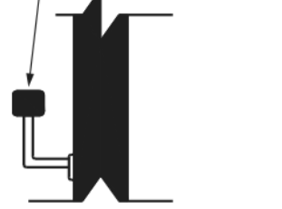
FIGURE 505.7(B) HANDRAIL CROSS SECTION - NONCIRCULAR
