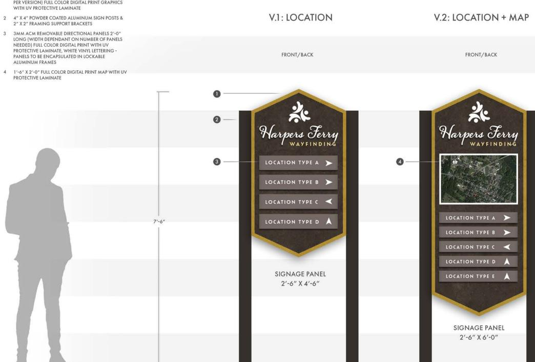
\*NOTE: SCALE SHOWN IS APPROXIMATED FOR CONCEPTUAL PURPOSES ONLY. APPROVED CONSTRUCTION DRAWINGS MAY IMPACT OVERALL DIMENSIONS.
